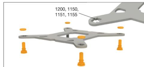
For fixing the backplate screws onto the Intel backplate use the O-rings. Once assembly of the Intel backplate for the respective Intel socket is complete, position it under the motherboard. In so doing make sure that the Intel backplate screws are precisely positioned inside the motherboard holes.
