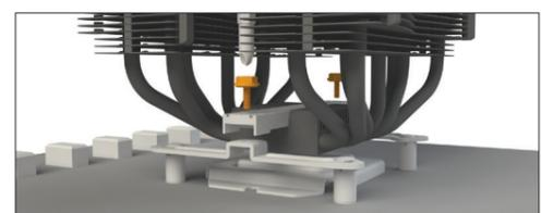
Fasten the Silent Wings 3 120mm fan using fan clips onto the front side of the cooler. Slide the 135mm fan between the two heatsinks and also fasten this with fan clips. Connect both fans using the the Y cable. Connect this to the CPU fan connector on the motherboard.
