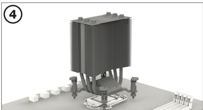
Place the cooler onto the CPU unit. Make sure that the Intel push-pins are precisely located within the motherboard holes.
