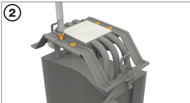
**Mounting the CPU cooler**
