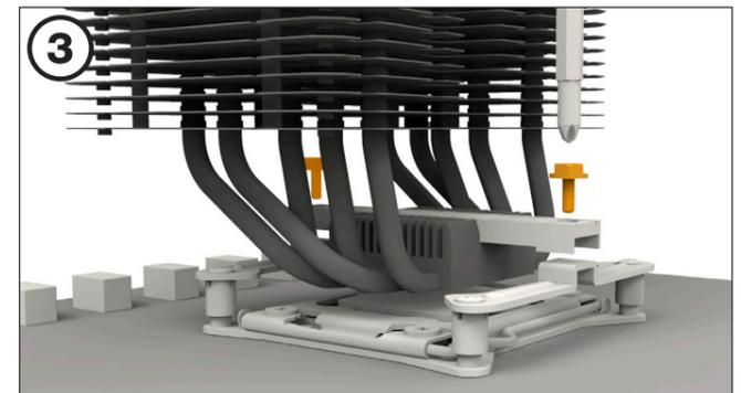
Position the cooler mounting bridge centrally on the cooler. Next place the cooler unit onto the CPU. Insert the mounting bridge fastening screws from above into the cooler mounting bridge and then screw these alternately tight.
