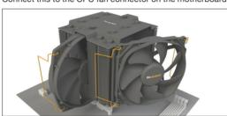
When dismantling the fans, push the notches of the fan clips (19) away from the fan.
