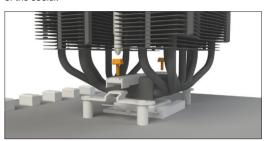
Fasten the Silent Wings 3 120mm fan (3) using fan clips (19) onto the front side of the cooler. Slide the 135mm fan (2) between the two heatsinks and also fasten this with fan clips (19). Connect both fans using the Y cable (20). Connect this to the CPU fan connector on the motherboard.
