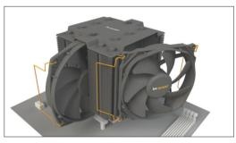
When dismantling the fans, push the notches of the fan clips
