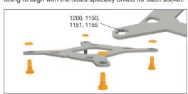
For fixing the backplate screws (14) onto the Intel backplate (4) use the O-rings (16). Once assembly of the Intel backplate (4) for the respective Intel socket is complete, position it under the motherboard. In so doing make sure that the Intel backplate screws (14) are precisely positioned inside the motherboard holes.
