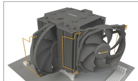
When dismantling the fans, push the notches of the fan clips (19) away from the fan.
