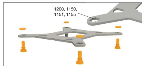
For fixing the backplate screws (14) onto the Intel backplate (4) use the O-rings (16). Once assembly of the Intel backplate (4) for the respective Intel socket is complete, position it under the motherboard. In so doing make sure that the Intel backplate screws (14) are precisely positioned inside the motherboard holes.
