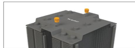
Position the cooler mounting bridge (8) centrally on the cooler (1). Next place the cooler unit over the CPU. Insert the Mounting bridge fastening screws (13) from above into the cooler mounting bridge (8) and then screw these alternately tight. You can use the cross-tip screwdriver (17) for this. Subsequently retighten both heatpipe caps on the top side of the cooler.
