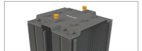
Position the cooler mounting bridge (8) centrally on the cooler (1). Next place the cooler unit over the CPU. Insert the Mounting bridge fastening screws (13) from above into the cooler mounting bridge (8) and then screw these alternately tight. You can use the cross-tip screwdriver (17) for this. Subsequently retighten both heatpipe caps on the top side of the cooler.
