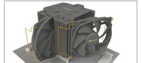
When dismantling the fans, push the notches of the fan clips (19) away from the fan.
